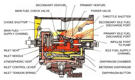
the fuel side of the metering diaphragm. Atmospheric air pressure on the opposite side will force the metering diaphragm upward causing the diaphragm button to contact the inlet control lever and overcome the inlet tension spring pressure, permitting fuel under pressure to force the needle off its seat and enter the metering chamber. The fuel then travels from the metering chamber up through the idle and main fuel supply orifices and channels and out the discharge ports to the engine.
